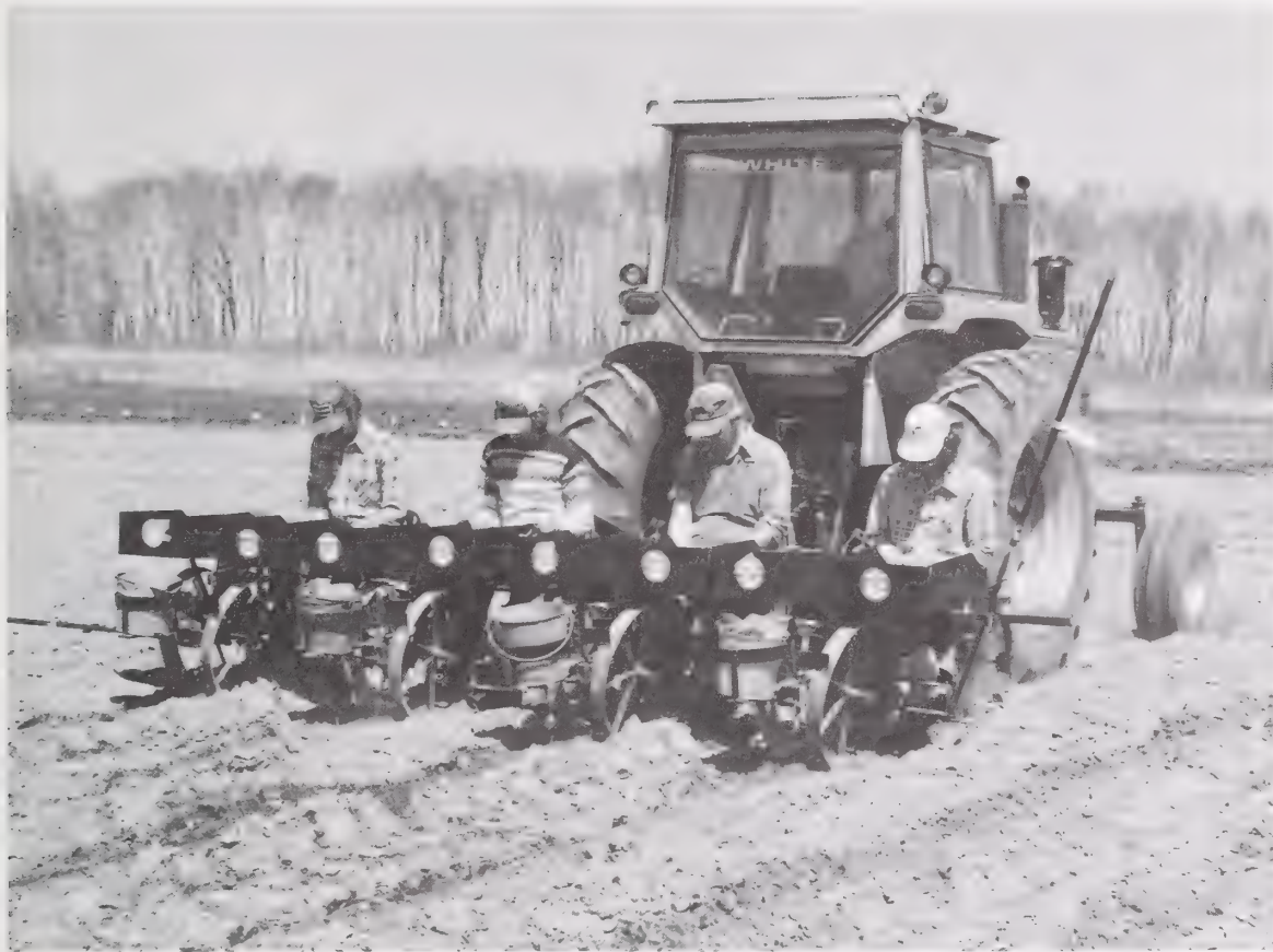
The machine digs the hole for the new tree seedling, the men drop the containerized seedlings into the hole and tamp them down with their feet, and the machine waters the seedlings before moving forward in the row. This system combines the best of both machine and hand planting.
